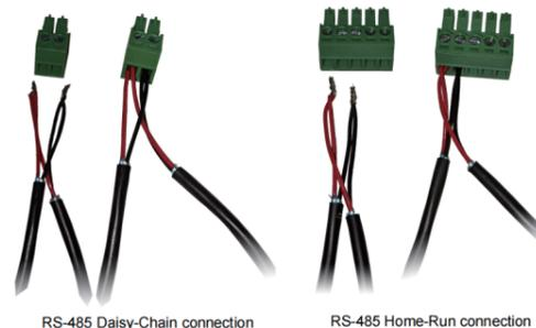
RS485 Control Output: RS485+ of PTZ camera connects to Ta of RS422 on the joystick controller and RS485 - of PTZ camera connects to Tb of RS422 on the Joystick controller.
