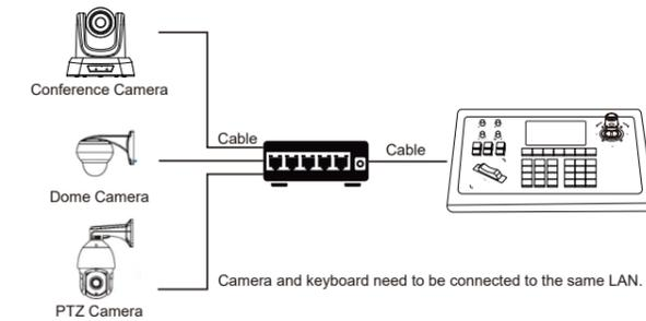
Connect the camera and joystick controller in the same LAN and ensure their IP address in the same network segment, such as 192.168.1.123 and 192.168.1.111 belong to the same network segment, while 192.168.1.123 and 192.168.0.125 do not belong to the same network segment, so you need to modify the joystick controller or the ptz camera IP address. The joystick controller gets its IP address dynamically.
